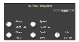
**Feedback:** Routes the processed signal back to the Module's input. Higher values create a sharper, more intense effect.
