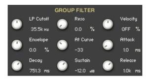
**LP/HP Cutoff:** Sets the frequency above which signals are attenuated. The Filter is a LP Filter when the knob is below zero and a HP Filter when the knob is above zero.
