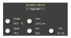
**Sync:** When Sync button is turned on, the Delay is synchronized to the external MIDI Clock.
