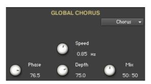
**Speed:** Sets the speed of the LFO modulating the signal.
