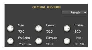
**Size:** Determines the room size by setting the length of the effect. Higher values simulate larger rooms, lower values smaller rooms.
