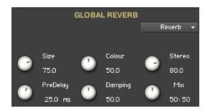
**Size:** Determines the room size by setting the length of the effect. Higher values simulate larger rooms, lower values smaller rooms.
