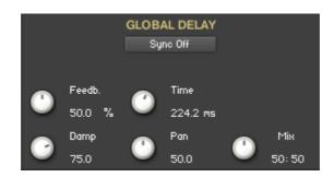
**Sync:** When Sync button is turned on, the Delay is synchronized to the external MIDI Clock.
