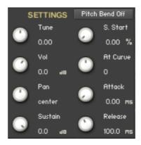
Here you can adjust all the various setting for the selected Key/Sound, like - **Tuning - Volume - Panning - Sample Start**.
