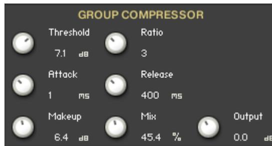
**Threshold:** Sets a level above which the compressor starts reducing peaks. Only signals above the threshold are affected by the compression ratio, signals below are unaffected.
