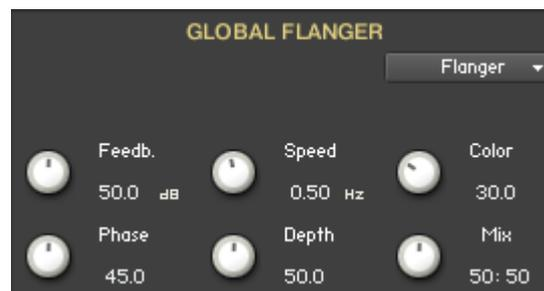
**Feedback:** Routes the processed signal back to the Module's input. Higher values create a sharper, more intense effect.
